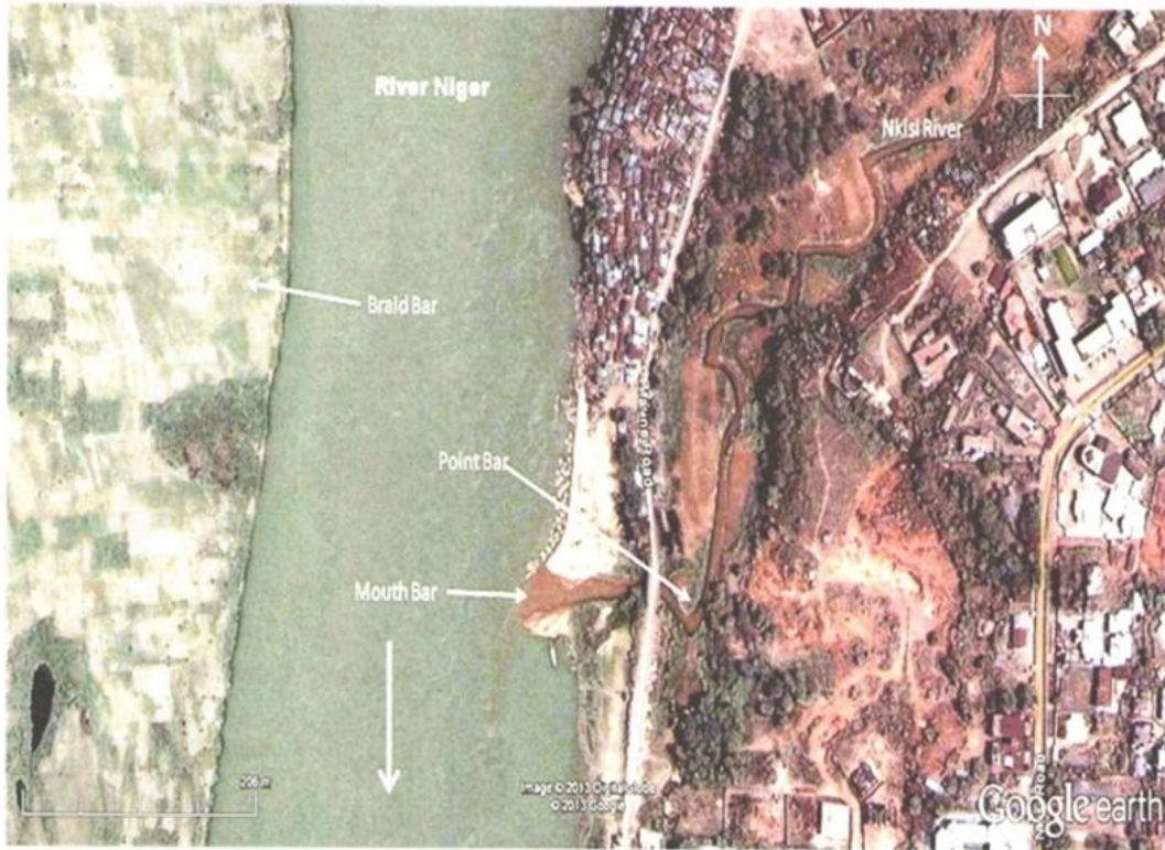
Fig. 2. River Niger showing braid bar, while Nkisi River showing point bar and mouth bar [14]
