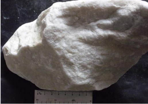
Plate 4a. Hand specimen of calc-gneiss at Lankpeshi mining site showing granular mineral texture
