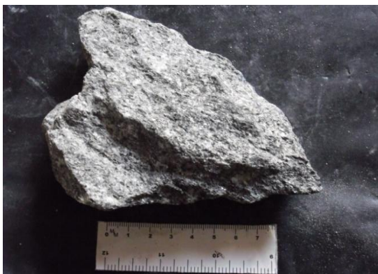
Plate 3a. Hand specimen of schist at Lankpeshi- Magongo Okene road showing grey colour and medium to coarse-grained texture
