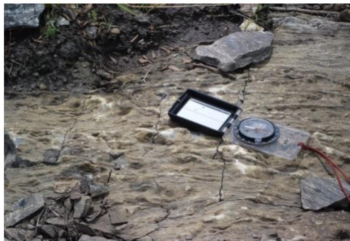
Plate 6. Field photograph of joints on schist at Lankpeshi mining site
