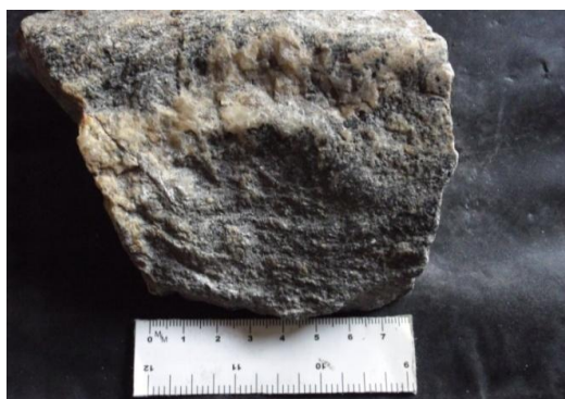
Plate 1a. Hand specimen of migmatite at Lankpesi- Magongo Okene road showing mixture of dark and light colour
