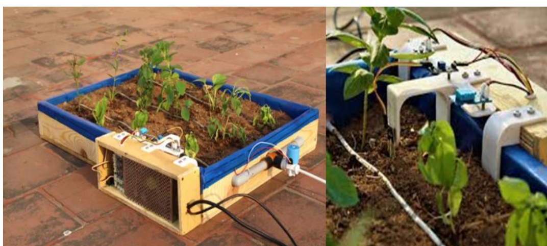
Fig. 3. Seed bed controlled by smart phone ( https://www.instructables.com/Raspberry-Pi-Powered-IOT-Garden/ )
