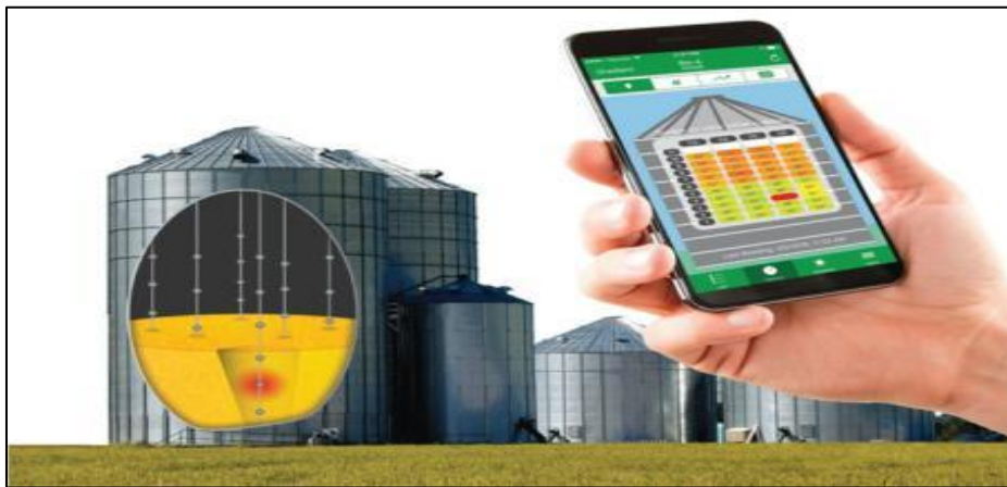
Fig. 7. Monitor seed storage with connected sensors (PC: https://www.tsgcinc.com/ )
