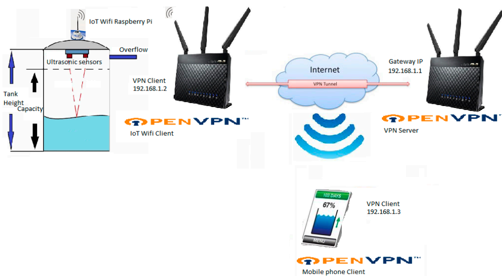
Figure 3. Pilot deployment of the proposed IoT security model for a smart water tank prototype.
