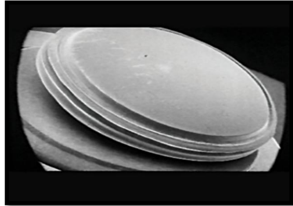
Fig. 1. Scanning electron micrograph of a Ridley intraocular lens made from PMMA
