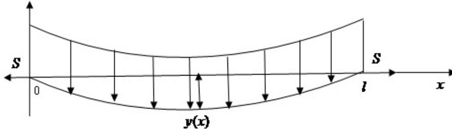
Fig. 1. Simply supported beam with a uniformly distributed load
